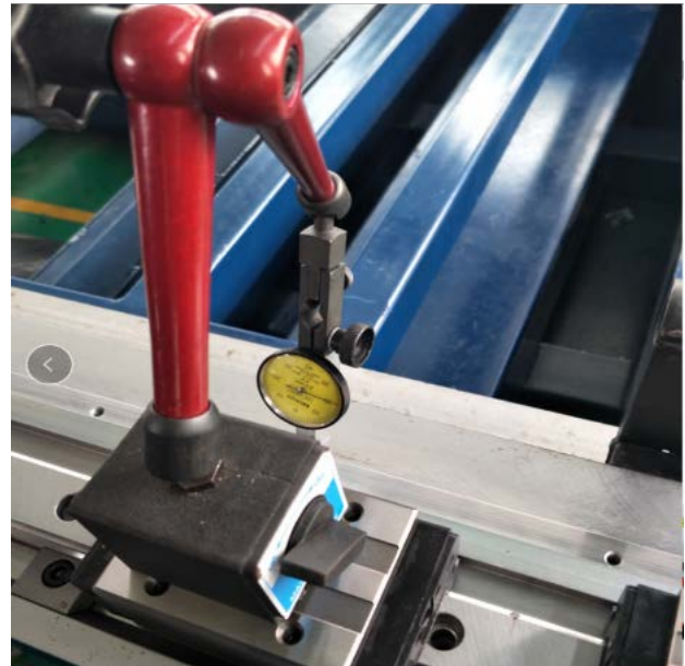
Linear guide parallelism examination, our requirement \leq \pm 0.02\text{mm}
