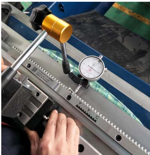
Guide gap detection, our requirements, our requirement \leq \pm 0.03\text{mm}
